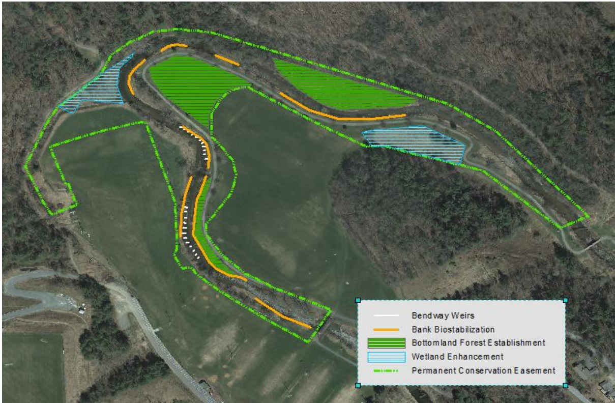
Fig 4 The overall site plan for the restoration. Primary restoration measures include rehabilitation of wetland areas, invasive species control and re-vegetation, riparian buffer extension and establishment, and bottomland hardwood forest re-vegetation as well as installation of bendway weirs.
